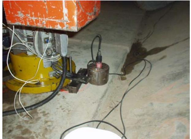
Fig. 2 Accelerometer on tunnel base
