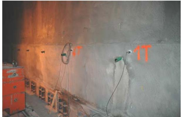
Fig. 3 Accelerometers on tunnel walls
