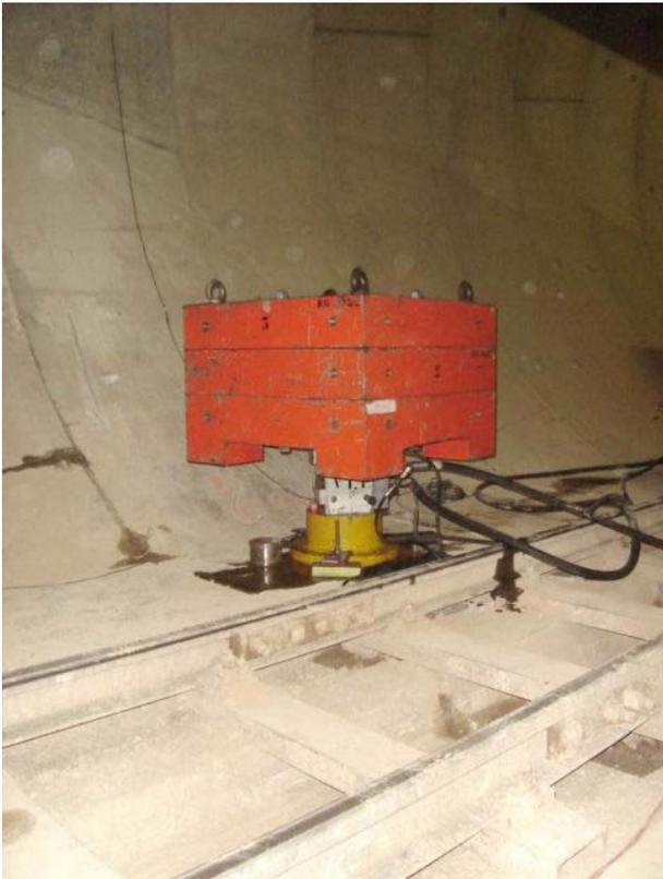
Fig. 1 Hydraulic exciter on the tunnel base
