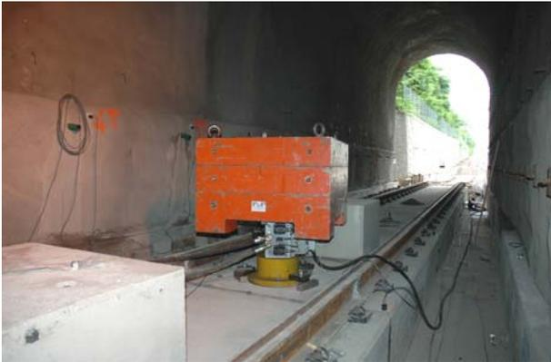
Fig. 12 – Vibrodyne on track and unsprung masses
