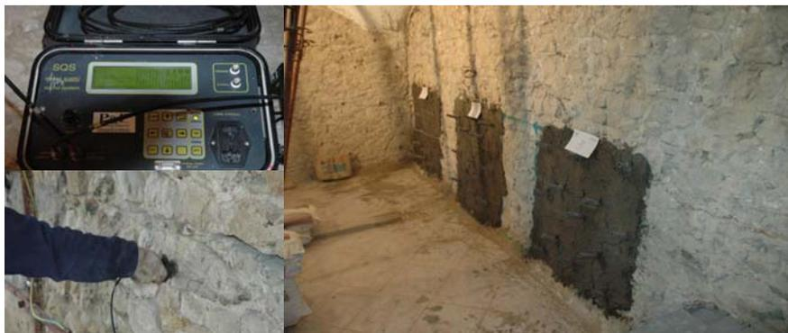
Figure 11. Sonic (left) and absorption (right) tests.
