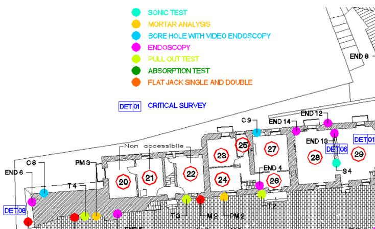
Figure 7. Examples of experimental tests on Marchesale Castle.
