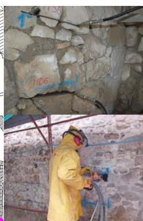
Figure 8. Flat jack tests.
