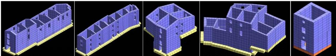
Figure 12. Simplified FEM of the whole structure.
